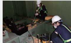
Sling rod load measurement
