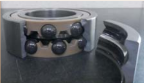
Damaged Bearing after Drop impact test
